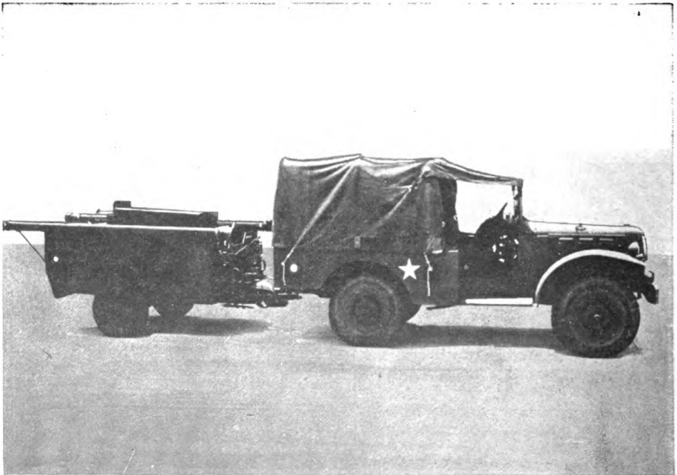
Figure 260. Trailer, fire, pumper, two-wheel, 500-g.p.m. class 1,000, complete with equipment.
